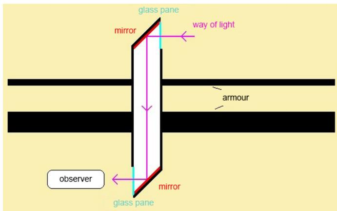
**Fig. 1.2** Schematic structure of a driver's optics
