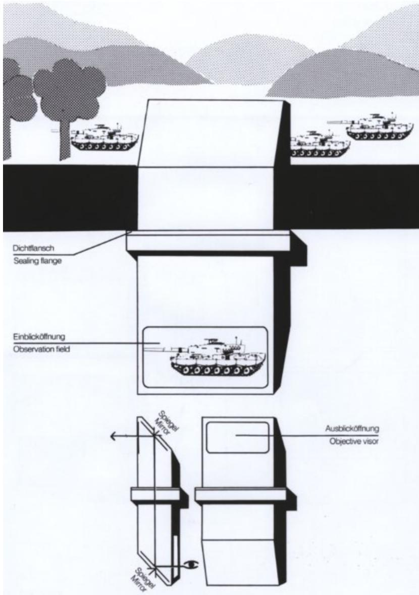
**Fig. 1.3** Design principle of a driver's optics
