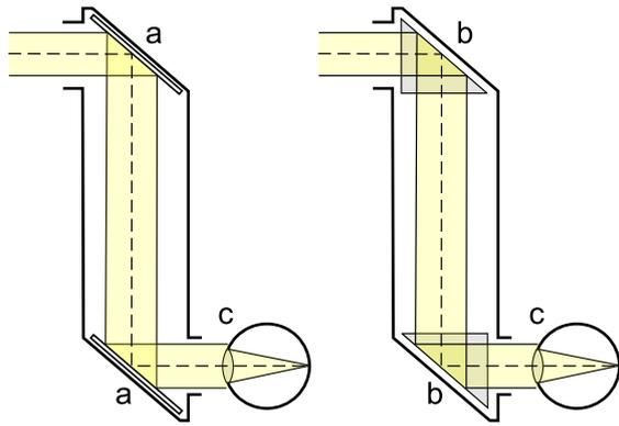
**Fig. 1.0** Periscope with mirrors (a) or deflecting prisms (b) and the respective observing eye (c)
